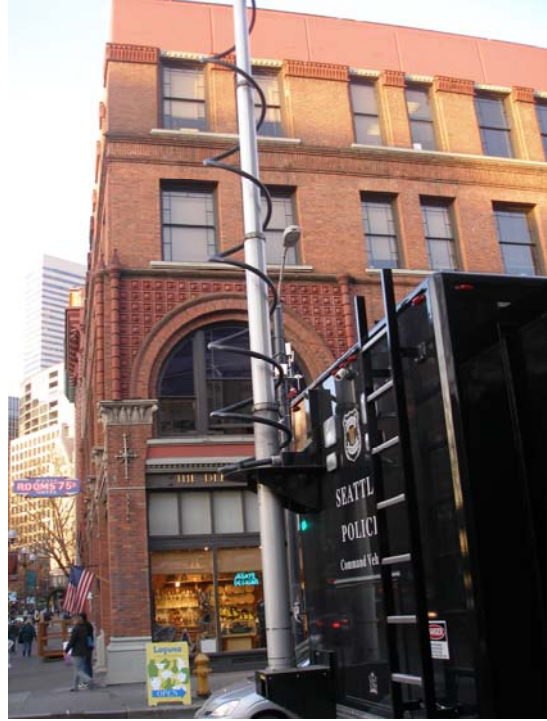
CAPTION: A quad-radio MSR4000 tri-band router receives video signals from nine cameras deployed over a 12-square-block area and centralizes them in the Seattle PD video surveillance center, where the video is then sent to provide views to a mobile police command center as well as handheld devices carried by individual patrolling officers.
