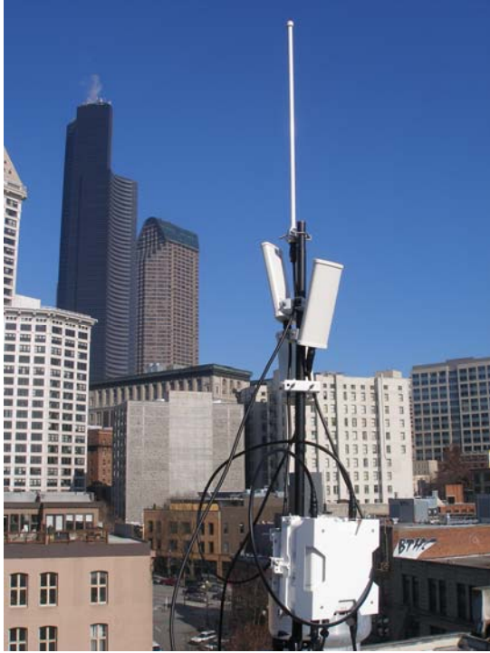
CAPTION: A quad-radio MSR4000 tri-band router receives video signals from nine cameras deployed over a 12-square-block area and centralizes them in the Seattle PD video surveillance center, where the video is then sent to provide views to a mobile police command center as well as handheld devices carried by individual patrolling officers.
